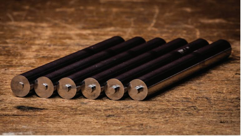
Temprel's **six-piece depth punch tool** set provides assurance that the thermocouples in the brake pad material are set to the appropriate depth. Correct use involves drilling a pilot hole into the test hardware and pressing the capped end of the thermocouple into place with the seating tool.
